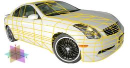
Make more polies around the details. Keep breaking down weird shapes into rectangles and then into triangles until you see nothing but triangles. Curved parts of the car will have more polies ofcourse.
