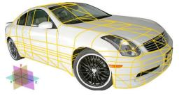
What about the non-rectangular components like the weird curves? Fill them in with multiple triangles!
